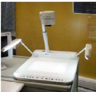
This device is used to transmit images and written material or other objects. Documents that are not in electronic format can be transmitted using the document camera.
