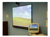
The Smart Board contains Smart Notebook software, which enables users to write information without space constraints. For example, math computations, chemical equations, derivation of theorems, etc., can be easily created using Smart Notebook and delivered using the Smart Board. The computer and Smart Board are used interactively.
