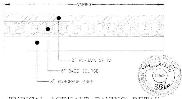
TYPICAL ASPHALT PAVING DETAIL
